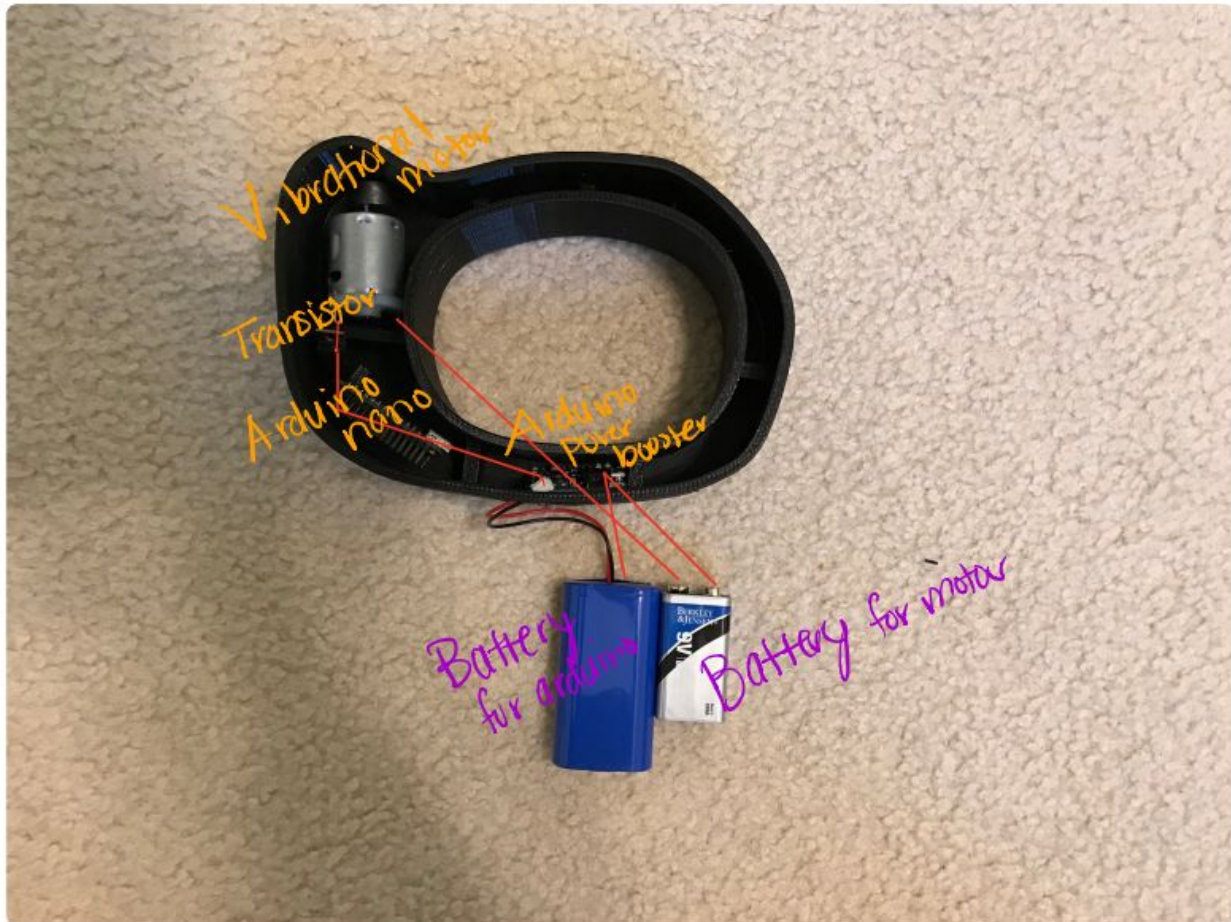
Figure 7.1.2.1 - Components fitted inside of handle
