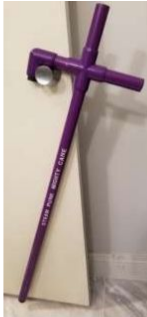
Figure 4.1.1.1 Non-adjustable Base of Previous Cane Design made using PVC
